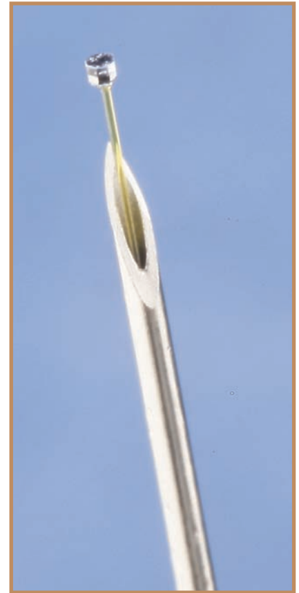
Figure 2. An FOP-MIV pressure sensor (here inserted in a 24-gauge hypodermic needle) is mass-produced by automated assembly lines. This 550- \mu\text{m} -outside-diameter optical sensor could be integrated into specialized catheters such as intra-aortic balloon (IAB) catheters, where it could provide EMI-free precise in situ blood pressure measurements used to trigger optimal balloon inflation/deflation during IAB pumping therapy. Courtesy of FISO Technologies Inc.
