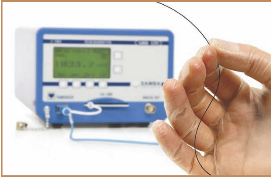
Figure 1. Samba Sensors' ultraminiature fiber optic pressure sensor is used to sense parameters including systolic blood pressure, intravascular blood pressure and intracranial pressure during trauma. Courtesy of Samba Sensors AB.
