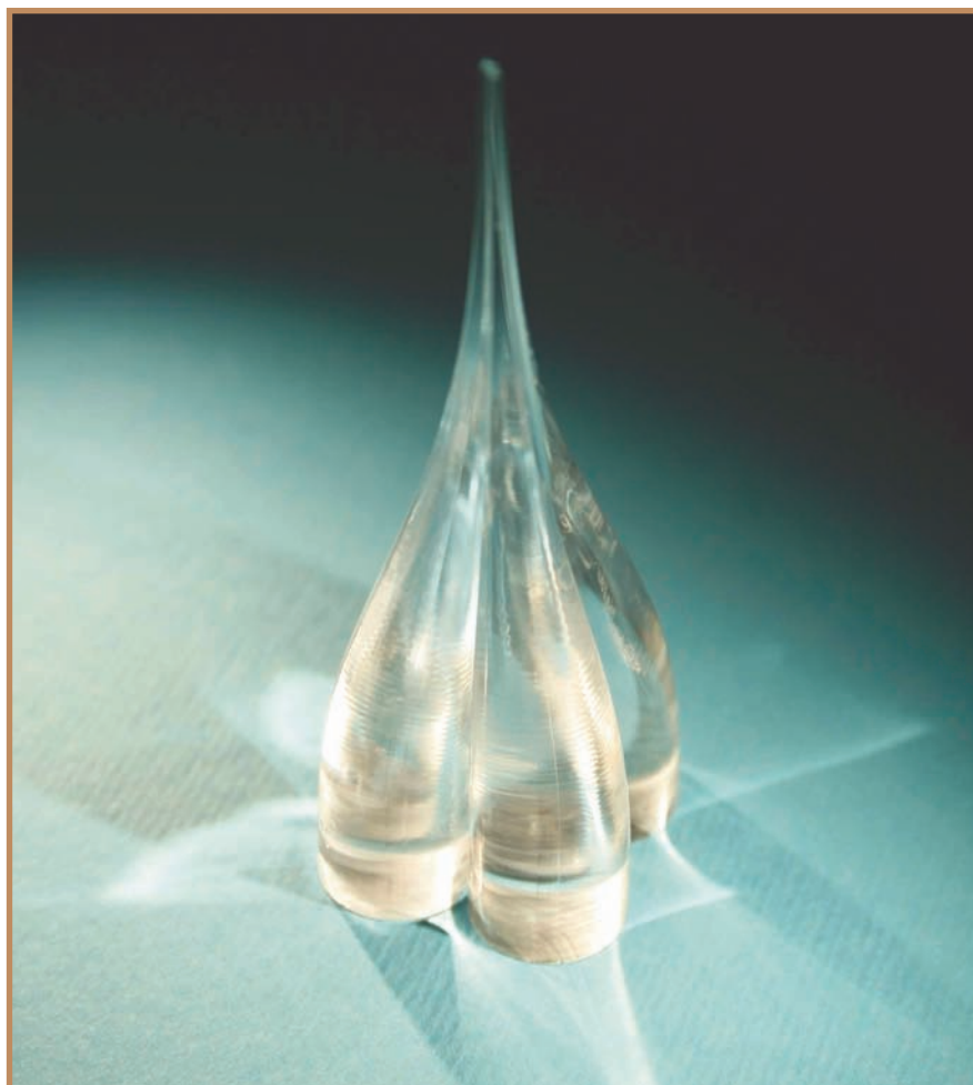
Figure 3. Gemini preform and drawn fiber. Courtesy of Acreo AB.
