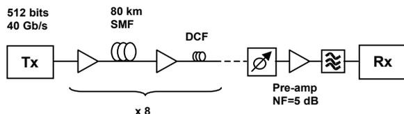
Fig. 1. The system considered in numerical simulations.
