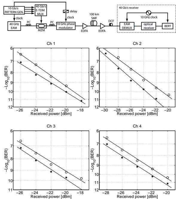
**Fig. 5.** Experimental setup (top) and BER vs. received power for all four TDM channels with (\*) and without (o) phase modulation (bottom).
