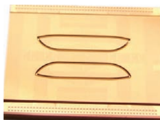
New chip design including microfluidic channels defined over four columns of silicon nanowires
