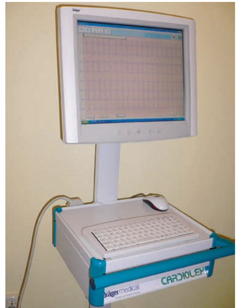
EKG system based on a standard PC
